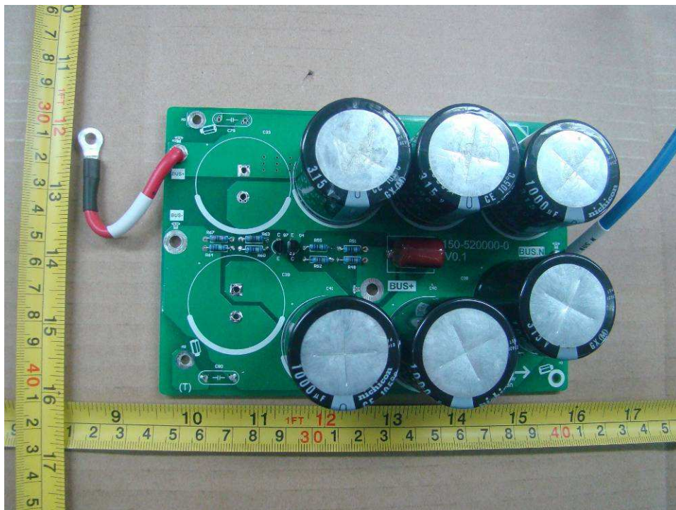
Cap board component side view SOFAR 3000TLM, SOFAR 3680TLM, SOFAR 4000TLM
